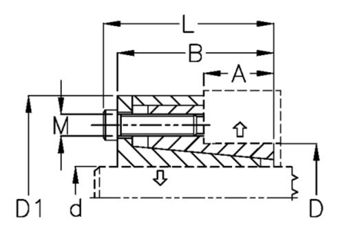
A mm = 27 B mm = 46.0 D1 mm = 70.5 d H8 mm = 38 D mm = 52 F kN torque = 44 L mm = 52.0 M mm = 6 P N/mm2 surface pressure on shaft/hub = 79
